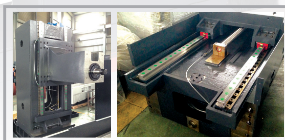
3 Axis use high rigid roller linear guide way provide accurate positioning and feeding Y axis and Z axis 45CA (block x 6) / X axis 55CA (block x 8)
