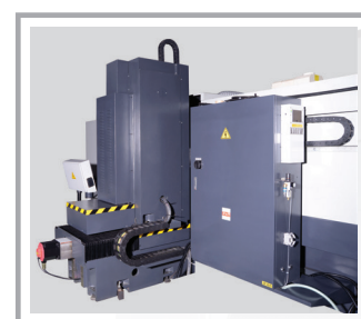
High rigid column (High rigid column design increase grinding stability)
