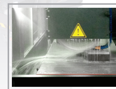
High pressure pump provides big water flow capacity during grinding
