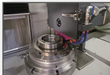
Horizontal Grinding Spindle for grinding surfaces and steps.
