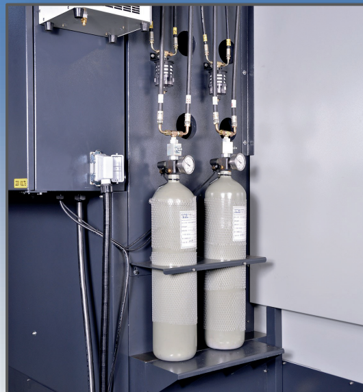
Nitrogen counterweight mechanism to reduce the screw and servo motor loading.
