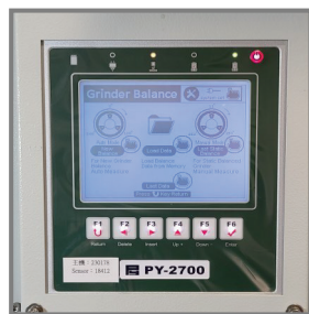
PY-2700 Balancer Online wheel balancing system. Measurable runout less than 1µm
