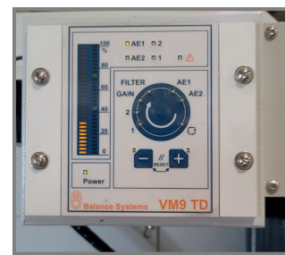
VM9 Touch Detector Detects wheel contact w/ workpiece or dressing post
