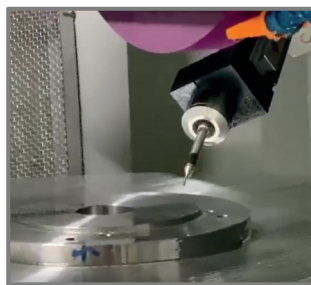
Renishaw LP2 Probe In process measuring accuracy of 2µm.
