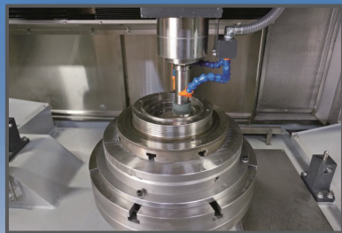
ID Grinding Spindle High-speed spindle can be refitted with different length arbors to achieve greater depths.
