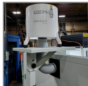
LOSMA Mist Collector Standard equipped on all machines with water tight enclosures
