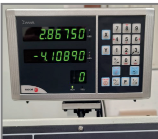
FAGO DRO For repeatable accuracy up to five place decimal.
