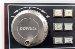
MPG hand wheel Graduations: 0.001, 0.005 and 0.01mm
